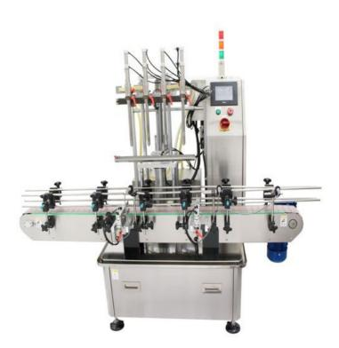
The Automatic Multi-nozzle Engine oil Pump High Speed Machine is designed to fill engine-oil-like liquid, lubricating oil, ...etc. Each nozzle equip with individual pump, making sure the stability. Diving nozzle to avoid foamy effect. Controlled by PLC, operated through HMI, memory set.
